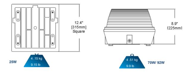
**INSTALLATION OPTIONS:** Standard fixture mounts to a flat surface using adjustable tabs or electrical j-box.
