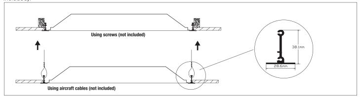
4.Place the kit in the ceiling opening and secure it with the screws.
