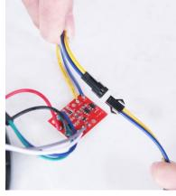
If lamp does not light as the above: Take apart the lamp cover Check circuit, if connector is dropping out , light on, then install. If there is no problem of the circuit, light is still not on, please pull up the connector and plug again then connect observation light If still not on, contact to custom service for treatment
