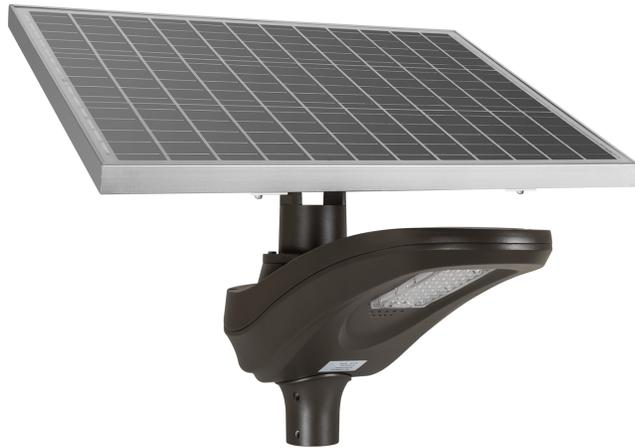
The working principle of solar LED street light: During the daytime, the solar street light is controlled by intelligent controller. The solar panel is irradiated by sunlight, absorbs the sun light and converts it into electric energy to charge the battery. At night, the battery pack provides power to supply the LED lighting to realize the illumination.
