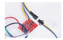
If lamp does not light as the above: Take apart the lamp cover Check circuit, if connector is dropping out, light on, then install. If there is no problem of the circuit, light is still not on, please pull up the connector and plug again then connect observation light If still not on, contact to custom service for treatment
