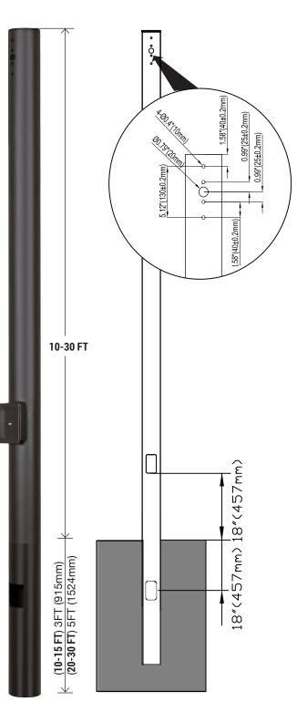
The Series Direct Burial Straight Round poles are built from high strength steel tube and are available side drilled for arm mounted area lighting luminaires or with tenon mounts for flood and post top luminaires. Typical area lighting applications include retail centers, industrial parks, schools and universities, public transit and airports, office buildings and medical facilities. Mounting heights of 10 to 30 feet can be used based on selected luminaire application.
