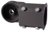
NEWT3SF2-D Slipfitter Mount An optional cast aluminum mast arm adapter secures fixture head to nominal 2"(2-3/8"O.D. pipe size) horizontal steel tenon arm.
