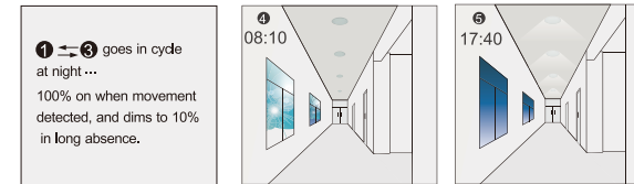
100% on when movement detected, and dims to 10% in long absence. When the natural light level exceeds setpoint off to light, the light will turn off even if when the space is occupied. The light automatically turns on at 10% when natural light is insufficient (no motion).
