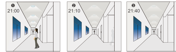
The light switches on at 100% when there is movement detected. The light dims to stand-by level after the hold-time. The light remains in dimming level at night.
