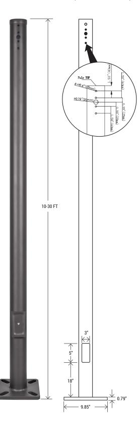
The Series Straight Round Steel poles are built from high strength steel tube and are available side drilled for arm mounted area lighting luminaires or with tenon mounts for flood and post top luminaires. Typical area lighting applications include retail centers, industrial parks, schools and universities, public transit and airports, office buildings and medical facilities. Mounting heights of 10 to 30 feet can be used based on selected luminaire application.
