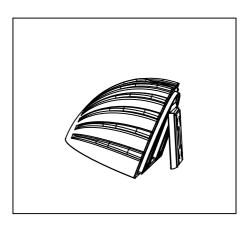
4) .After connected line, fitted with a reflector and PC cover, screw down the screws.
