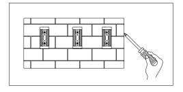
2.Drill the holes and screw on the bracket of the wall
