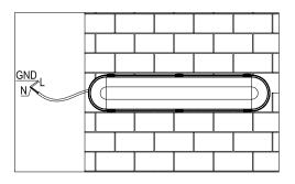
4. Connect the light to the electric supply,make sure the L/N/GND connect correct, use a waterproof connector if it is necessary.
