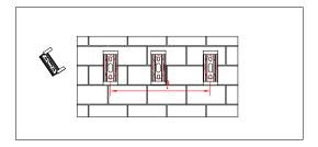
1. Mark on the wall the center of the lamp and the position of the two ends 63.78"(1620mm).
