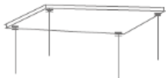
1. A. Fix the anchor into target place on the ceiling. B. Fix the installation mount on the ceiling with plastic anchor.
