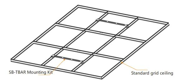
When Emergency led drivers can not be installed on the LED lights such as LED downlights, LED panel light & LED troffer. We can install the emergency led drivers on the Tbars and Tbars are installed on the grid ceiling.
